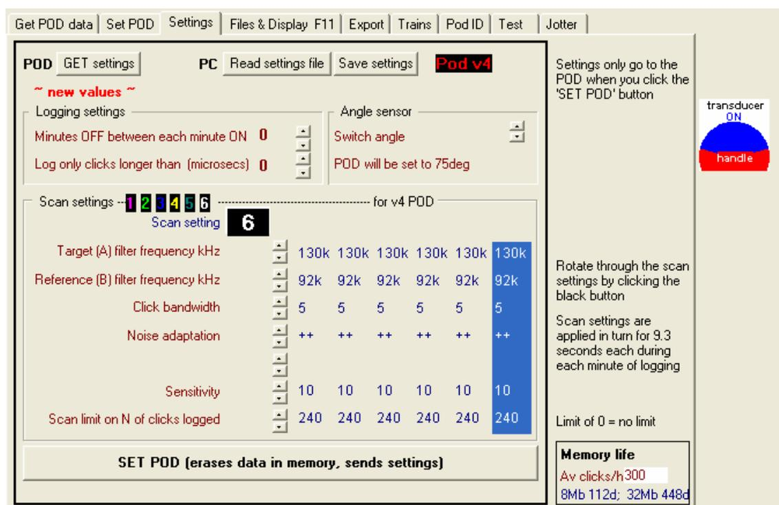
Fig. 5: Scan settings of the T-PODs. Sensitivity was set specifically for each T-POD.
