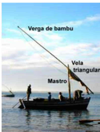
Figure 7: Schematic view of a lancha (from Santos, 2004)
