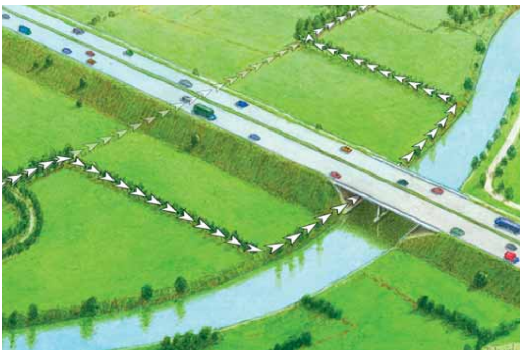
Figure 3: A spacious spanning of a watercourse with a bridge offers bats good possibilities to cross the road safely. Original hedgerows or tree lines can be rerouted to such a point
