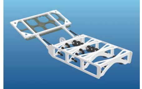
Example of job-specific tooling skid: Pipe tracking wheeled skid
