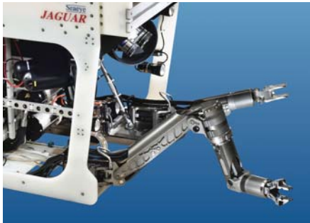
Jaguar fitted with Schilling Orion 7P and 4R
