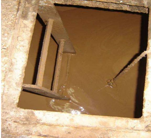
**Figure 13** Drilling mud in the respective reservoir
