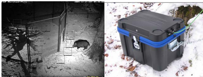
Fig. 2 Left : screen print of the black-and-white night lens of the digital video camera with motion detection windows (rectangles with dotted lines). These motion detection windows evaluate changes in pixel brightness between two succeeding live images. Right : weather-
